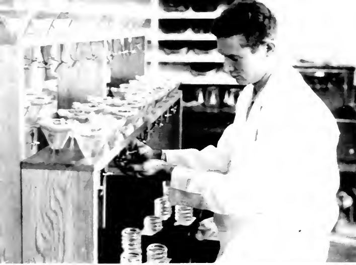
Extracting Plant Parasitic N From Soil, Using the Bou Funnel Technique
